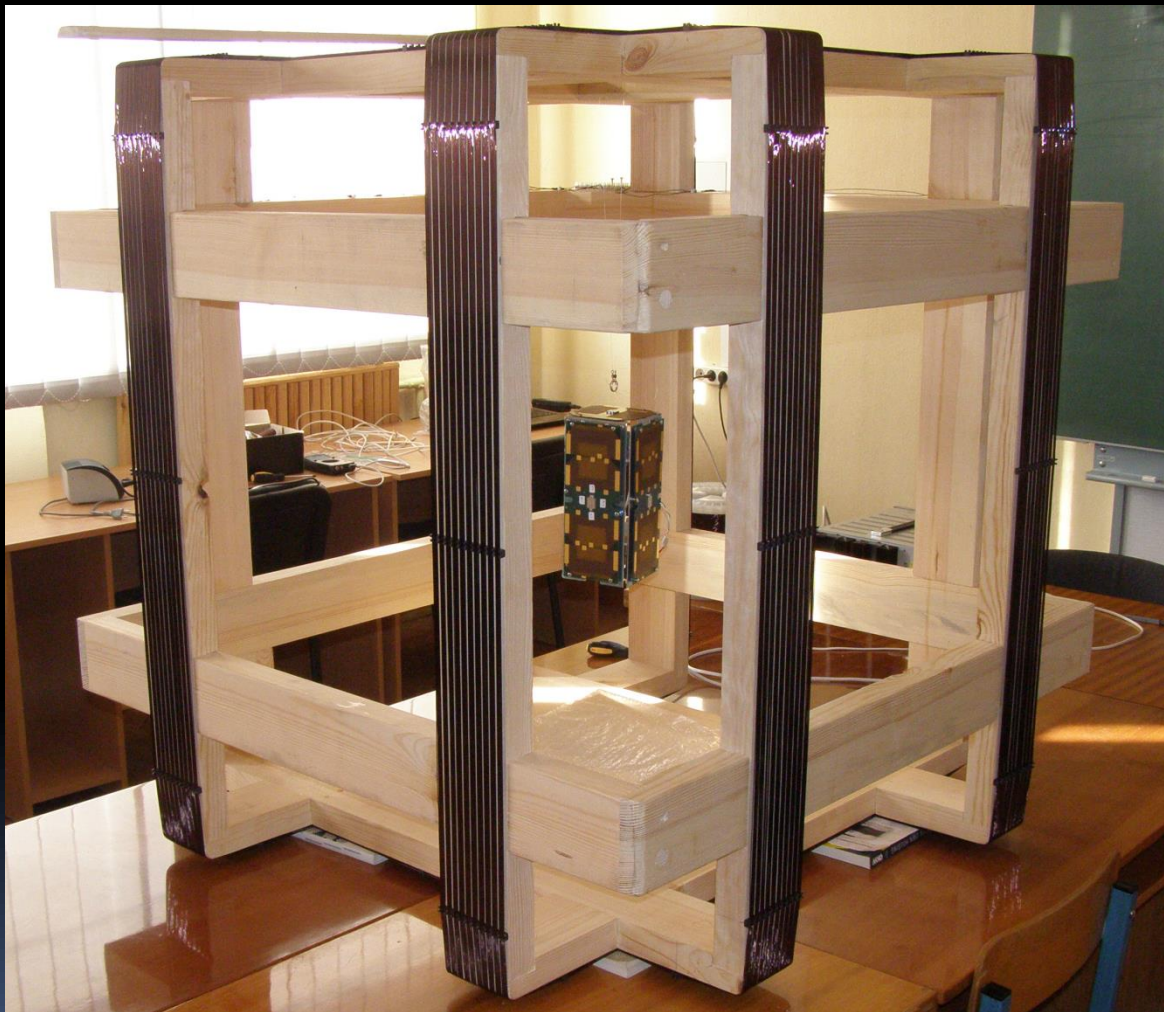
Magnetic induction field of the Earth \approx 50\text{mTl} , Coils reproduce magnetic field up to 300\text{mTl}
